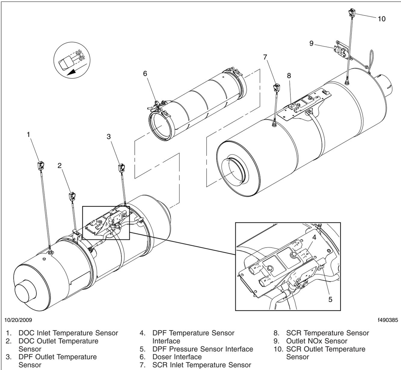
**Fig. 1, Cummins ATD Sensor Locations (inline ATS shown—design may vary)**
