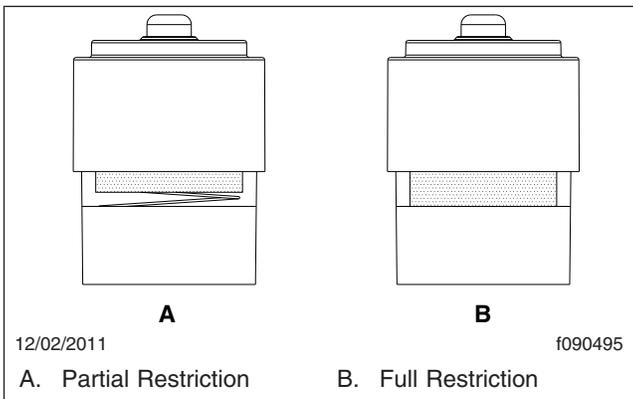
**Fig. 2, Air Restriction Indicator, Propane Engines**
