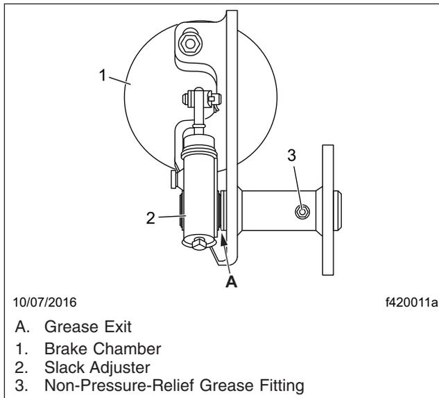
Fig. 6, Camshaft Bracket Lubricating
