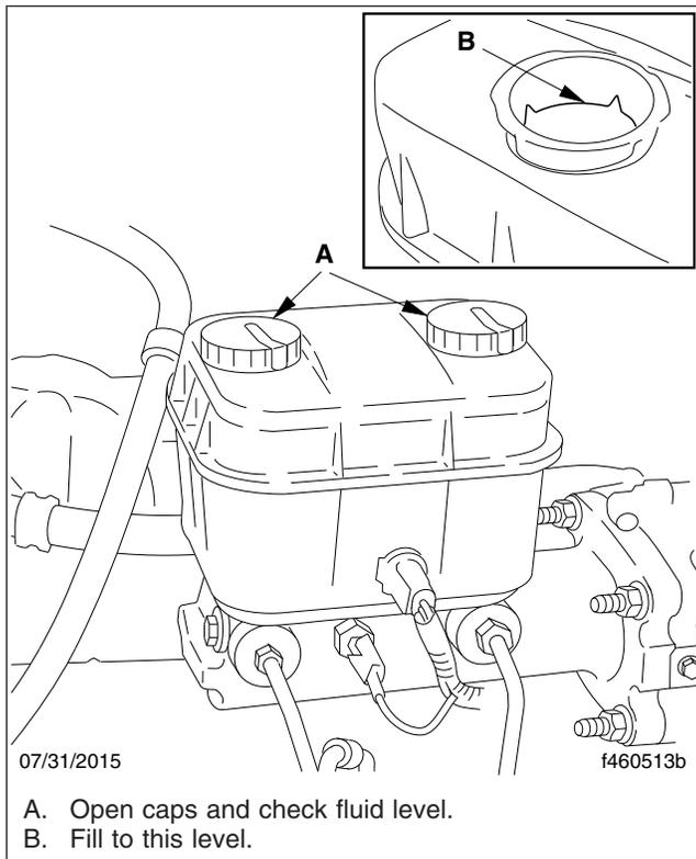
**Fig. 7, Hydraulic Brake Fluid Reservoir**
