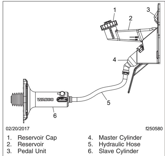
**Fig. 5, Clutch Components**
