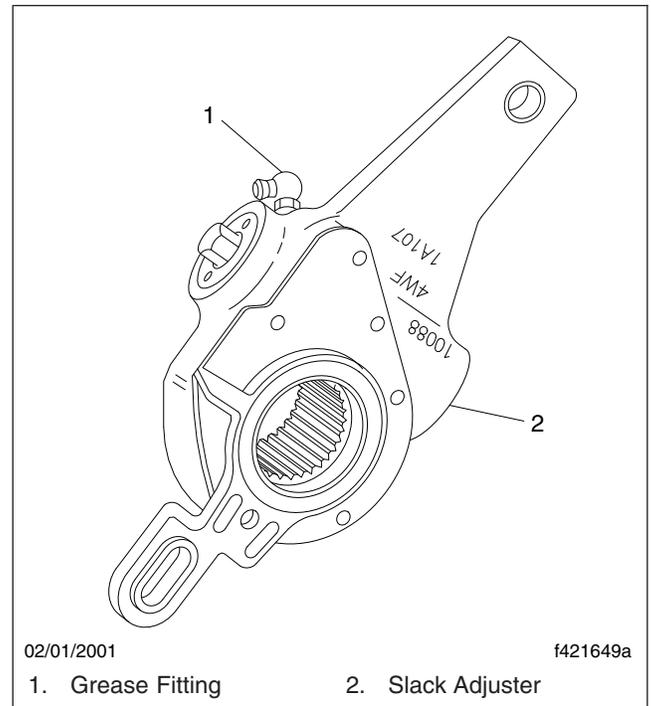
**Fig. 3, Haldex Slack Adjuster Grease Fitting**
