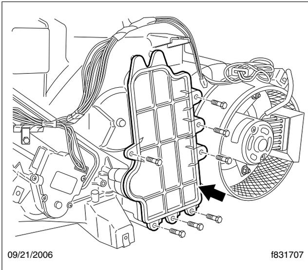
**Fig. 1, HVAC Cover Removal**
