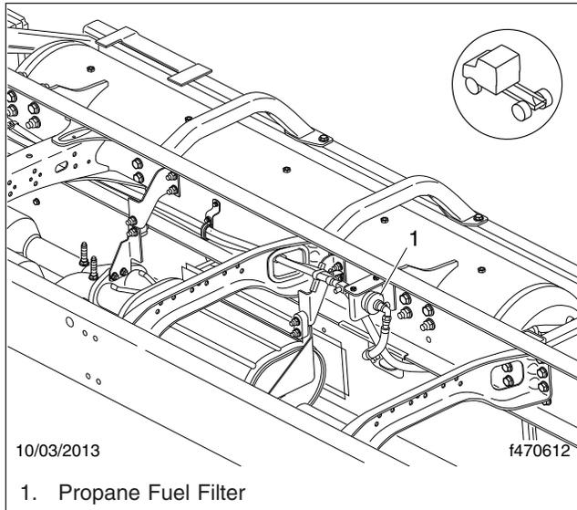
**Fig. 7, Fuel Filter Location (fuel going in the engine)**
