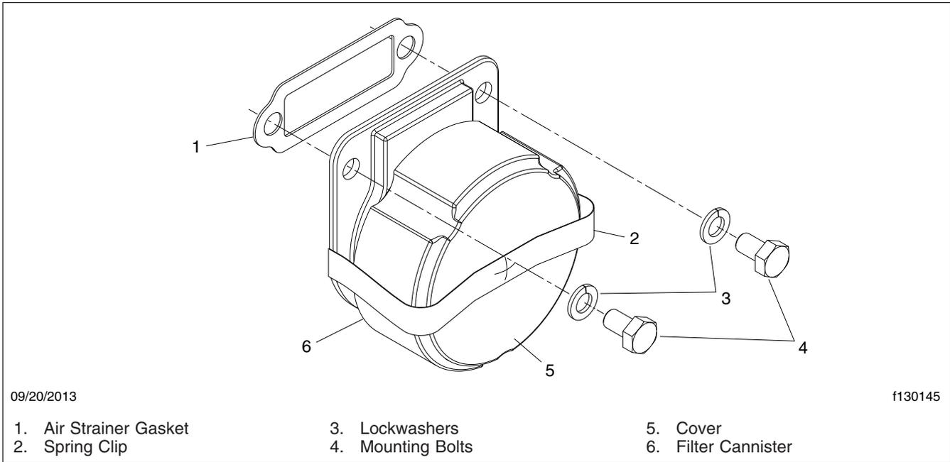
**Fig. 1, Pleated Paper Filter Assembly**
