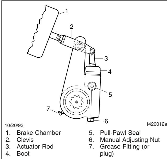
**Fig. 4, Meritor Automatic Slack Adjuster**
