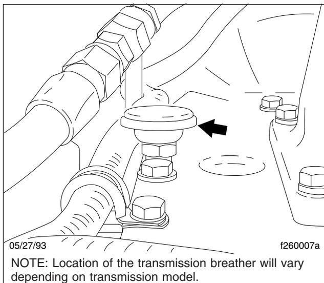
**Fig. 2, Transmission Breather (Eaton Fuller shown)**
