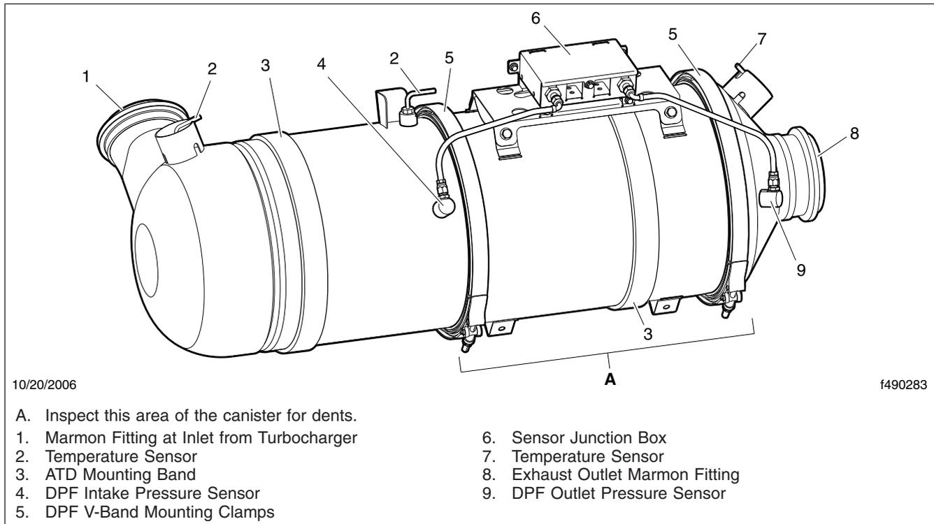
**Fig. 2, Typical Aftertreatment Device**
