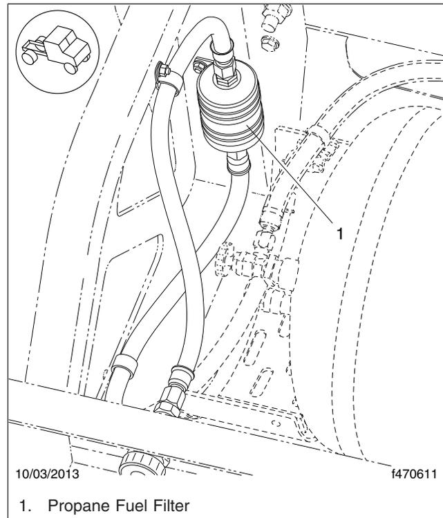
Fig. 6, Fuel Filter Location (fuel going in the tank)
