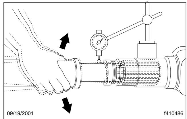
**Fig. 2, Checking for Radial Looseness of the Slip Yoke Spline**
