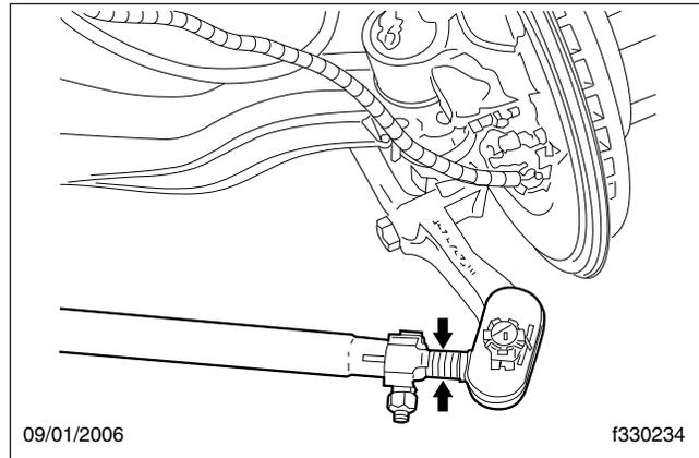
**Fig. 4, Checking Tie Rod End Movement**
