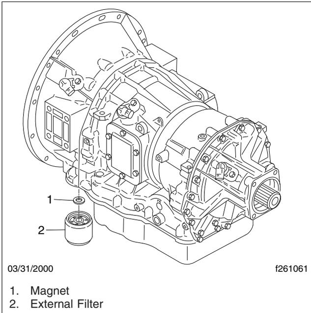
**Fig. 3, 2100/2200/2500 Series Transmission External Filter**
