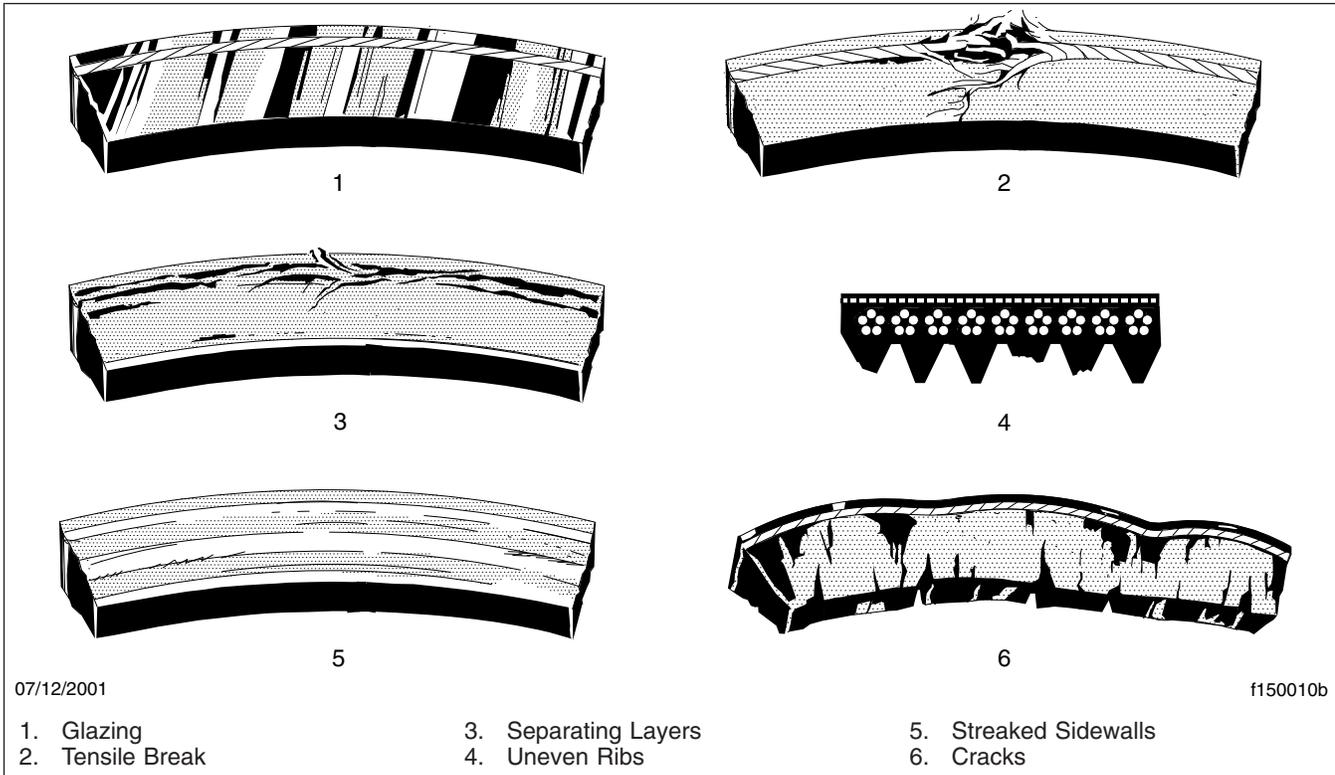
**Fig. 1, Drive Belt Replacement Conditions**
