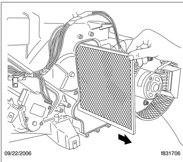
**Fig. 2, HVAC Assembly Filter Removal**
