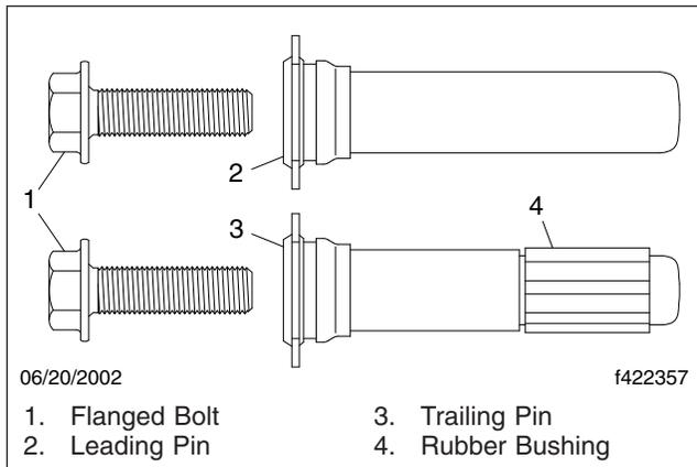
**Fig. 8, ZOH-T Slide Pins and Bolts**
