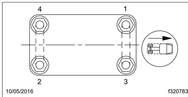
**Fig. 2, Tightening Sequence for U-Bolt High Nuts**
