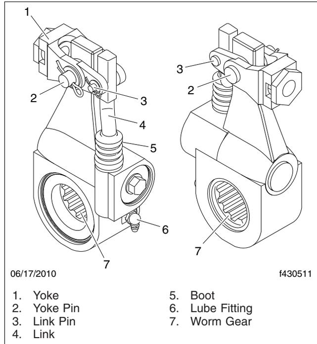
**Fig. 5, Bendix Automatic Slack Adjuster**
